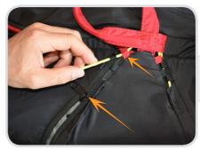
Feed both lower yellow plastics through their respective eyelets - always with the red eyelet first. Make sure both pins down each side of the container are correctly secured.
