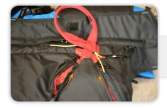
Run both container zips towards the reserve parachute handle, as far as they can go. Then reverse the direction of the zips to close the container. At this stage do not fully close the container, about half way is enough to secure the pin eyelets in position.
