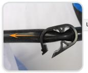
Unlock the stopper and remove it completely from the pipe.
