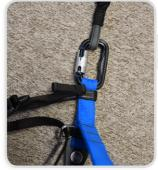
If you change the carabiners ensure that they are of a suitable dimension and fit correctly as shown
