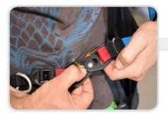
To undo the buckles first depress the red button and slide the buckle forward.
