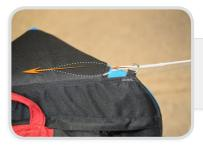
Feed the speed bar line through the metal ring and the opening of the protective sleeve - use a piece of plastic or magic line to pull the line through the protective sleeve. Then pass the line through the Ronstan pulley.
