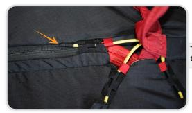
The end of the pin should be fed into the end pocket to fully secure it.
