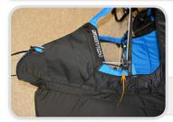
Attach the bar to the speed line and bungee using suitable knots. Once in the air, and when it is safe to do so, check that you can place your foot on the bar easily and that the system operates smoothly all the way to full speed.
