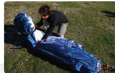
**Step 6.** Fold the wing with 3 or 4 folds whilst being careful to not crush the LE.
