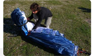
**Step 6.** Fold the wing with 3 or 4 folds whilst being careful to not crush the LE.
