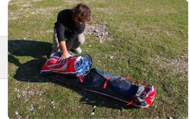
**IMPORTANT:** Do NOT lay the wing flat on the ground before packing the glider, this will cause abrasion damage to the top surface as you pull the glider towards the middle. ALWAYS pack from a mushroom or lift the wing off the ground when gathering the wing and grouping the leading edge.
