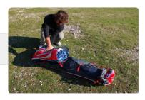
IMPORTANT: Do NOT lay the wing flat on the ground before packing the glider, this will cause abrasion damage to the top surface as you pull the glider towards the middle. ALWAYS pack from a mushroom or lift the wing off the ground when gathering the wing and grouping the leading edge.
