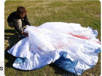
**Step 3.** Lay wing on its side and Strap LE...Note the glider is NOT folded in half; it is folded with a complete concertina from tip to tip. It is really important to not stress the middle cell or bend the plastic too tightly.
