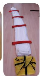
Keeping the lines neat and under tension, use figure of 8 folds and elastic bands around the loops to arrange the lines. The figure of 8s should be made to the same width as the deployment bag. Leave approximately 0.5m of line free at the end before the bridle.
