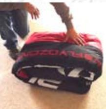
**IMPORTANT: Do NOT lay the wing flat on the ground before packing the glider, this will cause abrasion damage to the top surface as you pull the glider towards the middle. ALWAYS pack from a mushroom or lift the wing off the ground when gathering the wing and grouping the leading edge.**
