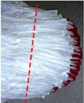
**Step 3.** Lay wing on its side and Strap LE...Note the glider is NOT folded in half; it is folded with a complete concertina from tip to tip. It is really important to not stress the middle cell or bend the plastic too tightly.
