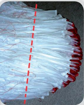
**Step 3.** Lay wing on its side and Strap LE...Note the glider is NOT folded in half; it is folded with a complete concertina from tip to tip. It is really important to not stress the middle cell or bend the plastic too tightly.
