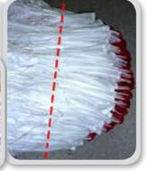
**Step 3.** Lay wing on its side and Strap LE...Note the glider is NOT folded in half; it is folded with a complete concertina from tip to tip. It is really important to not stress the middle cell or bend the plastic too tightly.
