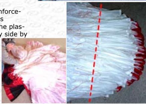
Step 3. Lay wing on its side and Strap LE...Note the glider is NOT folded in half; it is folded with a complete concertina from tip to tip. It is really important to not stress the middle cell or bend the plastic too tightly.
