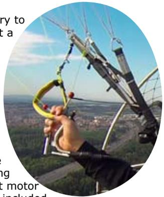
For directional control whilst flying at full speed only use the tip
