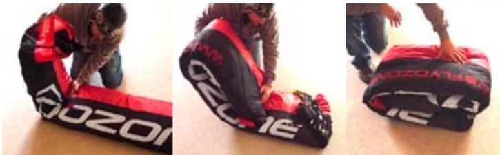
**IMPORTANT: Do NOT lay the wing flat on the ground before packing the glider, this will cause abrasion damage to the top surface as you pull the glider towards the middle. ALWAYS pack from a mushroom or lift the wing off the ground when gathering the wing and grouping the leading edge.**
