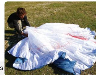
**Step 3.** Lay wing on its side and Strap LE...Note the glider is NOT folded in half; it is folded with a complete concertina from tip to tip. It is really important to not stress the middle cell or bend the plastic too tightly.
