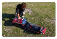
IMPORTANT: Do NOT lay the wing flat on the ground before packing the glider, this will cause abrasion damage to the top surface as you pull the glider towards the middle. ALWAYS pack from a mushroom or lift the wing off the ground when gathering the wing and grouping the leading edge.
