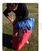
**Step 6.** Fold the wing with 3 or 4 folds whilst being careful to not crush the LE.
