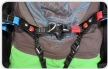
Ensure the buckles are closed properly, the red button should be up and the female buckles pulled fully so they are seated within the slots.
