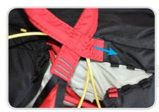
Now feed the reserve handle fully into the slot at the upper front part of the container. This secures the handle in position.
