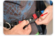
To undo the buckles first depress the red button and slide the buckle forward.
