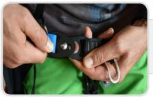
Fasten the leg/chest strap with the click buckles. The red button must be depressed to close and open the buckles. Slot the circular hole over the silver boss so that the red button is depressed and then slide the buckle backwards. The red button will pop up, the buckle is then locked in place.
