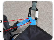
Attach the wing's risers to the carabiners at the main hang points. The A risers should be facing to the outside.
