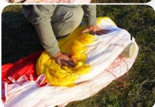
**Step 5.** Place the Folding Pillow below the LE - at the point of the first fold. The pillow reduces the angle of the fold and helps preserve the plastics. Next fold the TE over the LE being careful to not fold with tight angles.
