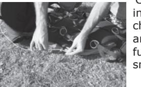
Ensure the speed bar lines are of equal length, double check that they are not too short as this may inadvertently activate the speed system when under tension in the air.
