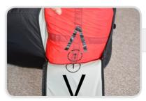
Place the deployment bag neatly within the container so that the ① and the arrow match those on the main flap. The parachute lines should be uppermost.
