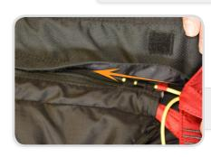
Now feed the yellow securing pins through the pin eyelets. Start with the pin located near the bridle. Each pin always starts with a red eyelet, feed the pin through each eyelet in order, there are four pins, make sure to not inadvertently miss any.
