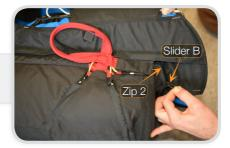
Carefully remove the upper parachute pin 1 being careful to not open the remaining pins.
