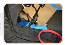
Do the same with the elastic bungee and tie to the pulley attachment loop using a suitable knot.
