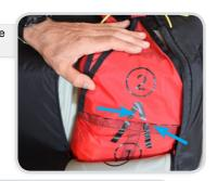
Slide the black tag of the handle between the bridle and harness to hold it in position.
