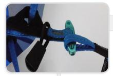
Fasten the leg/chest straps with the lightweight T lock buckles. Slip the T lock completely through the loop and then secure in place with the elastic loop.
