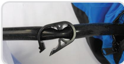
Make sure the stopper is in the open position and attach the inflation pipe to the outlet found on the stuff sack.
