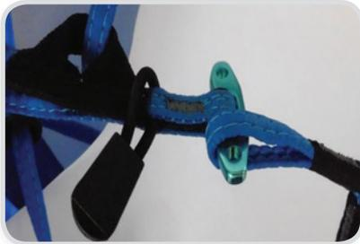
Fasten the leg/cheat straps with the lightweight T lock buckles.
