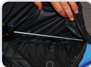
Ensure that the lines run cleanly through the pulleys and pass to the outside of all structural webbing straps.
