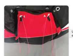
Using suitable pieces of magic string or plastic, pull the white loops through the parachute container evelets.
