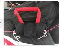
Now the top flap can be pulled into position. The handle sits behind the exterior material of the top flap. Pass the nylon pins of the reserve handle through the gaps in the material just above the top flap eyelets.
