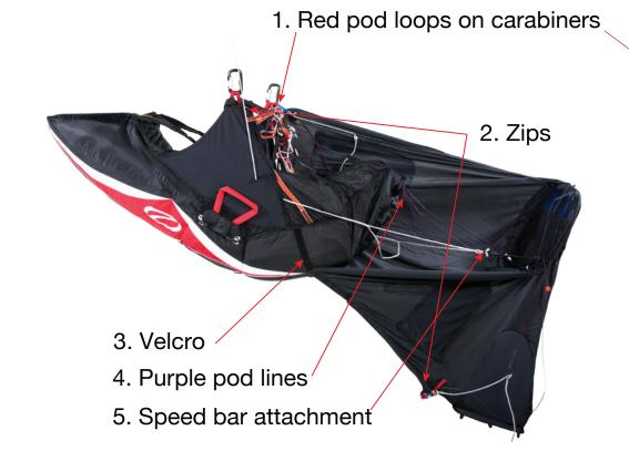
IMPORTANT: Ensure the red pod loops (1) are attached to the carabiners. Failure to do so will put excessive load through the zip causing failure.
