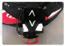
Pay attention to the bridles. Do not allow them to become entangled, they should remain neatly in place to the left hand side of the parachute when inserting.
