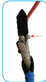
Double check the Link Lite is closed correctly, it should look exactly as shown.
