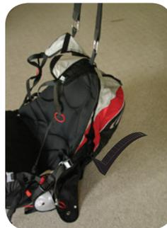
Maillons must be closed tightly - finger tight then 1/2 a turn with pliers is sufficient. Do not overtighten.
