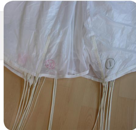
**4** Now prepare the panels and lines neatly. Using a parachute line spacer helps with this stage but is not mandatory.
