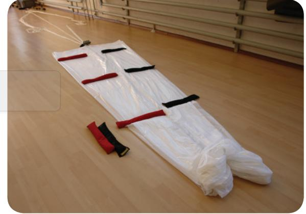
**8** Completely fold the gores of one side over to the other so that all of the gores are on top of each other.
