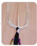
Organise the gores by folding each one individually over to one side, counting as you go. The Angel 90/95/110 have 18 gores and the Angel 140 has 20. The gores are numbered in red and black at the skirt of the parachute near to the line attachment points. Sort the parachute so that half of the gores are to each side of the double apex lines with gore number 1 and either 18 (90/95/110) or 20 (140) clearly identified on top.
