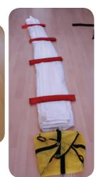
Keeping the lines neat and under tension, use figure of 8 folds and elastic bands around the loops to arrange the lines. The figure of 8s should be made to the same width as the deployment bag. Leave approximately 0.5m of line free at the end before the bridle.
