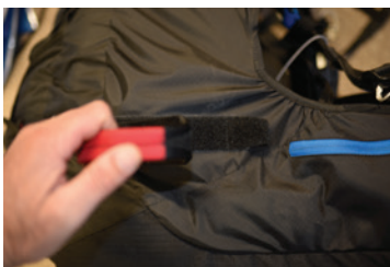
As part of the daily check, remove and replace the handle several times.
