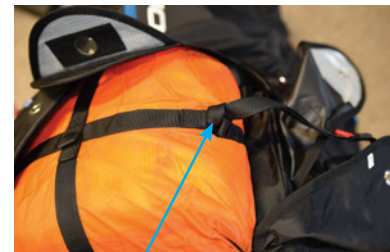
It is advised to attach the deployment handle to the loop on the side of the deployment bag.
