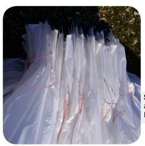
**Step 2.** Group leading edge (LE) plastic reinforcements with the A tabs roughly aligned. Make sure the plastic reinforcements lay side by side. Note the glider is NOT folded in half; it is folded as a complete concertina from wing tip to wing tip.
