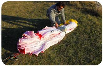
**Step 4.** Once the LE and TE of the wing have been sorted, turn the whole wing on its side.
