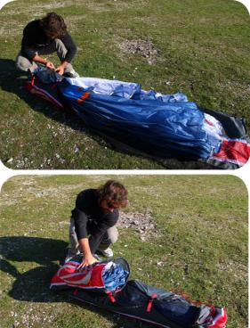
**IMPORTANT:** Do NOT lay the wing flat on the ground before packing the glider, this will cause abrasion damage to the top surface as you pull the glider towards the middle. ALWAYS pack from a mushroom or lift the wing off the ground when gathering the wing and grouping the leading edge.
