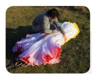
Step 3. Group together the middle and the trailing edge (TE) of the wing by sorting the concertina folds near the B and C tabs.
