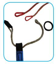
Continue pulling the B loop through the risers/lines/ring for the second turn.
