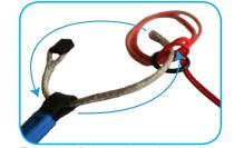
Feed the B loop through the riser, then through the line loops, passing behind the lines before going through the riser for the second time. Tension the Link Lite so it is approximately the correct dimension, the A tab should be close to the risers.
