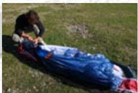
**Step 8**. Turn the Saucisse on its side, lay the foam Folding Pillow in place and make the fold of the LE around it. Use 3 folds.
