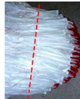
Step 3. Strap LE...Note the glider is NOT folded in half; it is folded with a complete concertina from tip to tip. It is really important to not stress the middle cell or bend the plastic too tightly.
