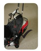
Maillons must be closed tightly - finger tight then 1/2 a turn with pliers is sufficient. Do not overtighten.
