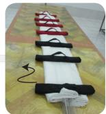
Now arrange the lines keeping them neat and under tension. Use figure of 8 folds and elastic bands around the loops to arrange the lines neatly. The figure of 8s should be made to the same width as the deployment bag. Leave approximately 0.5m of line free at the end before the bridle.
