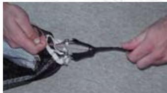
Ensure that the central line is not in the disabled position. Do this by pulling the disabling line through the bridal.
