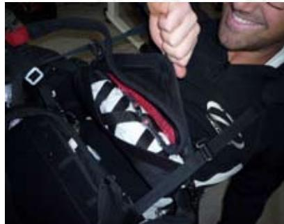
Put both brakes into one hand and open the deployment bag.
