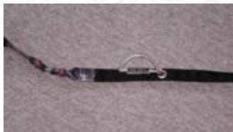
Midway along the bridle, just beyond the swivel is the centre line handle (3). Pulling this kills the power of the parachute and allows you to make your landing approach.
