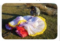
Step 2. Group leading edge (LE) plastic reinforcements with the A tabs roughly aligned. Make sure the plastic reinforcements lay side by side. Note the glider is NOT folded in half; it is folded as a complete concertina from wing tip to wing tip.
