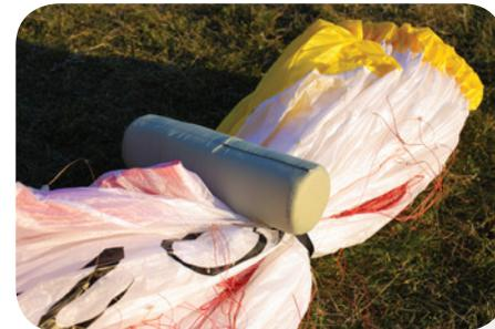
**Step 5.** Strap the Folding Pillow below the LE - at the point of the first fold. The pillow reduces the angle of the fold and helps preserve the plastics. Next fold the TE over the LE being careful to not fold with tight angles.
