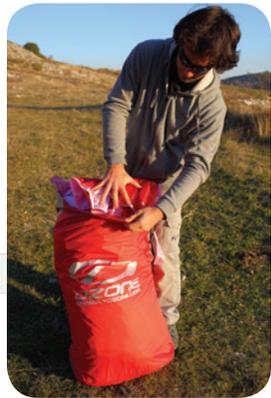
**Step 7.** If using a Saucisse, with the wing laid on its side carefully close the zip (or clips) without trapping any material.
