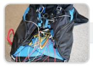
Ensure all the buckles, carabiners, risers and structural straps are placed on the inside of the harness structure, then fold the harness in half so the parachute is uppermost.
