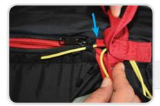
Now feed the yellow securing pins through the pin eyelets. Start with the pin located near the bridle. Each pin always starts with a red eyelet, feed the pin through each eyelet in order, make sure to not miss any inadvertently.
