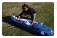
Step 5. Once the LE and rear of the wing have been sorted, turn the whole wing on its side.
