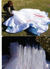
Step 4. Group together the middle/trailing edge of the wing by sorting the folds near the B, C and D tabs.
