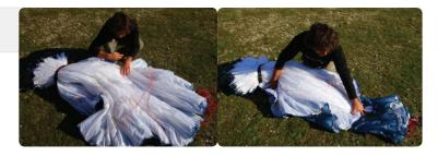
Step 5. Once the LE and rear of the wing have been sorted, turn the whole wing on its side.
