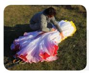
**Step 3.** Group together the middle and the trailing edge (TE) of the wing by sorting the concertina folds near the B and C tabs.
