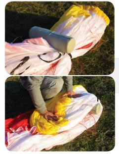
**Step 5.** Place the Folding Pillow below the LE at the point of the first fold. The pillow reduces the angle of the fold and helps preserve the plastics. Next fold the TE over the LE being careful to not fold with tight angles.
