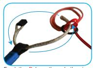
Feed the B loop through the riser, then through the line loops, passing behind the lines before going through the riser for the second time. Tension the Link Lite so it is approximately the correct dimension, the A tab should be close to the risers.
