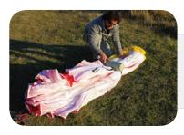
Step 5. Strap the Folding Pillow below the LE - at the point of the first fold. The pillow reduces the angle of the fold and helps preserve the plastics. Next fold the TE around the LE being careful to not fold with tight angles
