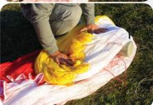
**Step 5.** Place the Folding Pillow below the LE - at the point of the first fold. The pillow reduces the angle of the fold and helps preserve the plastics. Next fold the TE over the LE being careful to not fold with tight angles.
