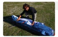
**Step 5.** Once the LE and rear of the wing have been sorted, turn the whole wing on its side.
