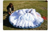
**Step 3.** Lay wing on its side and Strap LE...Note the glider is NOT folded in half; it is folded with a complete concertina from tip to tip. It is really important to not stress the middle cell or bend the plastic too tightly.
