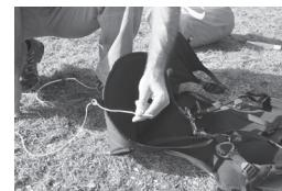
Ensure the speed bar lines are of equal length, double check that they are not too short as this may inadvertently activate the speed system when under tension in the air.
