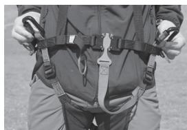
**Chest strap** – The maximum setting is 44cm which is ideal for most pilots and is the distance Ozone recommends. It is possible to reduce further by tightening the strap in the air.
