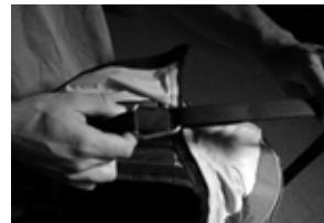
1. Attach harness bridles to the hang points located at the shoulders using suitable karabiners. Make sure that the bridles are untwisted and fit neatly into the Velcro bridle protection sleeve.
