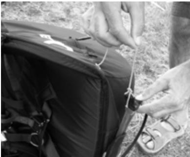
Attach the speed bar with a Bowline knot.
