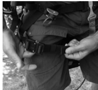
Leg straps should be adjusted whilst in a standing position so that they are not too loose and not too tight. If the leg straps are too loose you will find it difficult to rotate into the seated position after take off. If they are too tight you will find it difficult to run, they may also cut off circulation to your vitals!
