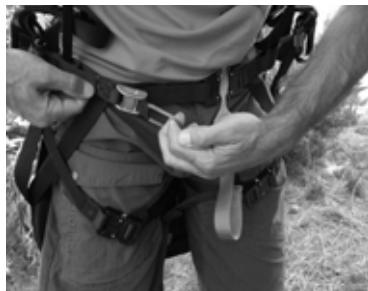
It is possible to adjust by tightening or releasing the strap in the air but it is safer to make these adjustments on the ground in small increments as only small adjustments have a significant impact to the feel in flight. For less roll and less glider feedback tighten the chest strap, for more roll response and more glider feedback release the adjustment tab. Please refer to the manual supplied with your glider to verify certified harness settings.
