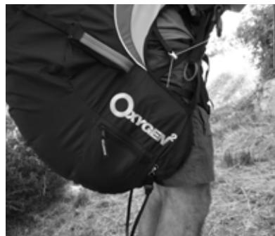
If you are restricted from standing up straight, then the shoulder straps are too tight, release the tabs until the edge of the seat plate sits just above the knee. It is normal for the shoulder straps to be slightly loose whilst seated in flight.
