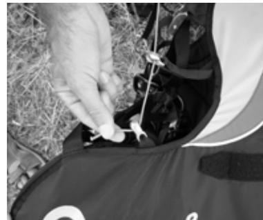
To fit a speed bar, route the lines through the two pulleys and the eyelet on each side of the harness.
