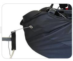
Double-check all the lines, check they run freely and have not been inadvertently wrapped around any of the structural webbing.
