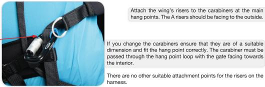
Attach the wing's risers to the carabiners at the main hang points. The A risers should be facing to the outside.
