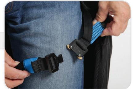
Connect the chest strap T lock buckles once again ensuring there is an audible click each time and slide the free end of the chest strap protector into the sleeve.
