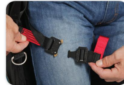
Fasten the colour coded leg straps, ensure there is an audible click and that they are properly secured.
