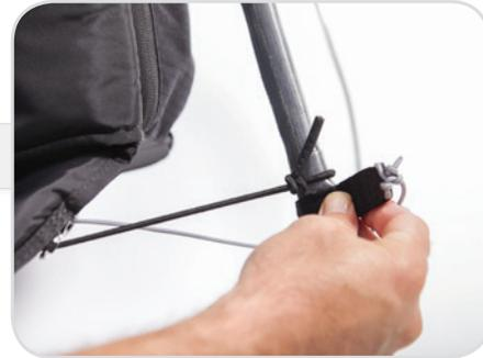
Now set the length of the speed bar. This is best done on a static hang point or alternatively it can be done on the ground. Make sure the speed system is not set too short and that it is symmetrical.
