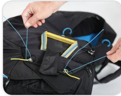
Now the top flap can be pulled into position. The handle sits behind the exterior material of the top flap and is secured with Velcro. Pass the nylon pins of the reserve handle through the gaps in the material just above the top flap eyelets. Pull the white loops through both top flap eyelets (D and 4) and push the pins through the white loops.
