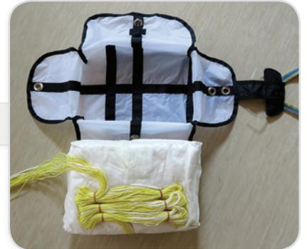
Insert the parachute into the deployment bag and secure the deployment bag with the lines in the normal way. Depending on the size of your parachute you can use any of the eyelets for the best fit.
