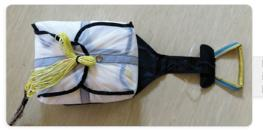
Insert the parachute into the deployment bag and secure the deployment bag with the lines in the normal way. Depending on the size of your parachute you can use either eyelet for the best fit.
