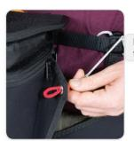
Next pass the red loop of the anti-forget system through the eyelet on the right hand pod next to the instrument panel.
