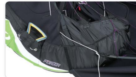
Ensure that the lines run cleanly between the pulleys and pass on the outside of all structural webbing straps. Double-check the lines have not inadvertently wrapped around any of the structural webbing straps. Attach the speed bar with a Bowline knot and repeat the procedure on the other side.
