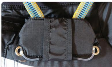
Finally the ends of the nylon pins can be neatened into the available tunnel as shown.
