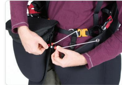
The red ball found under the left hand maillon should now be passed through the loop of the anti-forget system.
