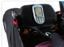
The Cockpit is integral to the pod, instruments can be attached either directly to the cockpit or alternatively to the additional angled Velcro plate. In the air it rests over the top of the chest strap to make it easy to view the instruments.
