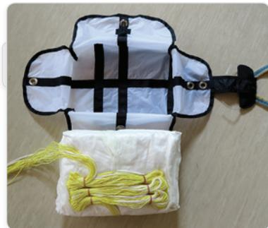
To install a reserve parachute you should first pack the parachute so that it matches the shape and dimension of the supplied deployment bag.
