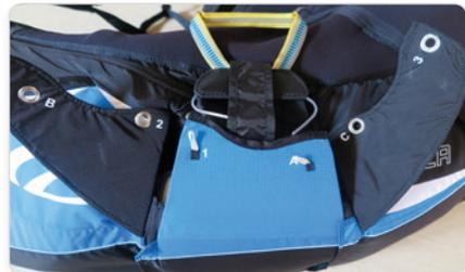
Gently pull the parachute handle and top flap out of the way so they are clear of the bottom flaps
