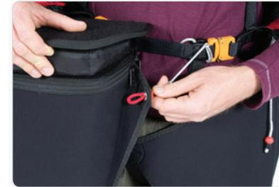
Next pass the red loop of the anti-forget system through the eyelet on the right hand pod next to the instrument panel.
