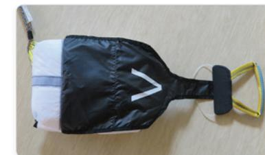
Open the reserve parachute container on the rear of the harness by opening the zips. Place the deployment bag in the space provided with white arrow on the deployment handle facing uppermost so that it matches the white arrow on the harness, the parachute lines should be underneath and the handle positioned correctly as shown.
