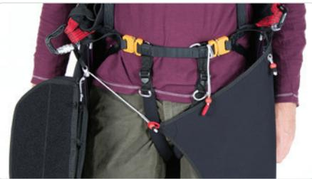
The automatic pod closing system should now be connected. First attach the red loop of the left hand pod flap to the red ball situated under the maillon on the right hand side of the harness. The red ball goes through the red loop.
