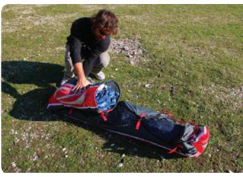
**IMPORTANT:** Do NOT lay the wing flat on the ground before packing the glider, this will cause abrasion damage to the top surface as you pull the glider towards the middle. **ALWAYS** pack from a mushroom or lift the wing off the ground when gathering the wing and grouping the leading edge.
