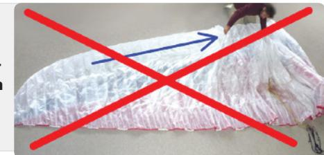
**IMPORTANT:** Do not fold the glider in the centre, you will bend the plastics, instead pack the wing with a full concertina method from tip to tip before packing into the stuff sac.
