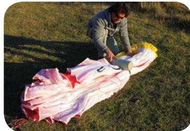
**Step 5.** Strap the Folding Pillow below the LE - at the point of the first fold. The pillow reduces the angle of the fold and helps preserve the plastics. Next fold the TE around the LE being careful not to fold with tight angles
