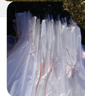
**Step 4.** Group together the middle/trailing edge of the wing by sorting the folds near the B, C and D tabs.
