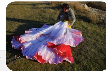
**Step 3.** Lay wing on its side and Strap LE...Note the glider is NOT folded in half; it is folded with a complete concertina from tip to tip. It is really important to not stress the middle cell or bend the plastic too tightly.
